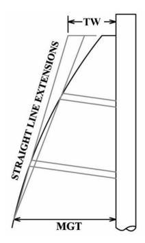
**10.29.2 MGT, MGU, MGM and MGL** shall be the length of the widths of the mainsail taken at points 7/8, 3/4, 1/2 and 1/4 of the leech from the clew respectively, measured in accordance with 10.28.
