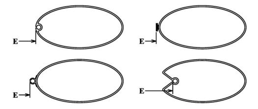
**2. Sheeting Limit (BAL)**. BAL shall be the distance from the outer measurement point of E to a contrasting measurement band denoting the limit on the boom beyond which no lead for the sheeting of headsails shall be attached. In the absence of such a band BAL shall be measured to the boom end. BAL shall not exceed 0.152 m (0.50 ft.).
